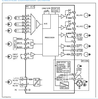
Transmitter temperature monitoring with programmable high/low alarm
